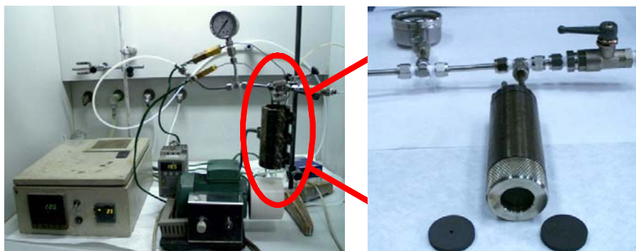
Figure 5.1. Fibre-maker equipment (left). In more detail, fibre spinning device (right) with spinnerets.
