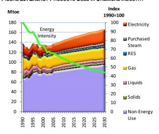
The energy in the chemical industry is mainly used in thermal processes. Thermal use concerns mainly steam, which account for 45% of total energy consumed for energy purposes in the sector. Specific thermal processes account for 25%, the rest being covered by electricity.
